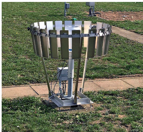
rain[e]H3 and windshield in use at DWD
